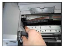
Ensure the length of tube so that the cartridge can thoroughly move to Both sides.
